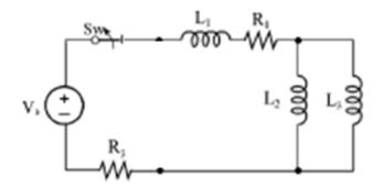
The switch stays closed.  $L_1 = 20 \text{ }mH$ ,  $L_2 = 40 \text{ }mH$ ,  $L_3 = 60 \text{ }mH$ ,  $R_1 = 22 \Omega = R_2$ . Let  $V_s = 10 \text{ }V$ .
